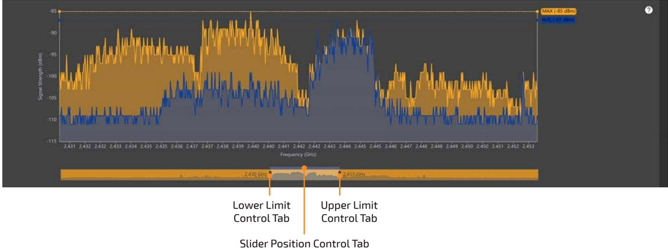
This range can be moved up and down the spectrum by clicking and dragging the slider position control tab.
