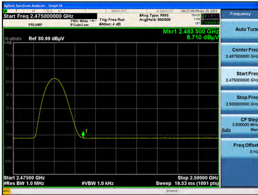
Radiated Restricted Band Edges plot – Average Reading ( \pi/4 DQPSK, Ch.78, X-V)
