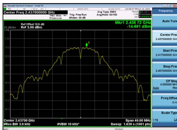
Power spectral density-802.11g ,2412MHz
