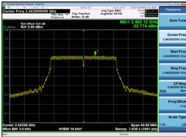
Power spectral density-802.11n(HT20) ,2462MHz
