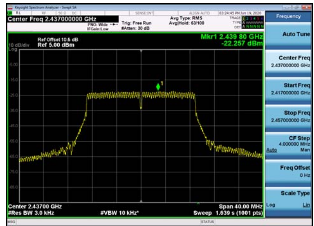
Power spectral density-802.11n(HT20) ,2437MHz
