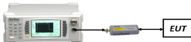
Figure 7-3. Test Instrument & Measurement Setup
