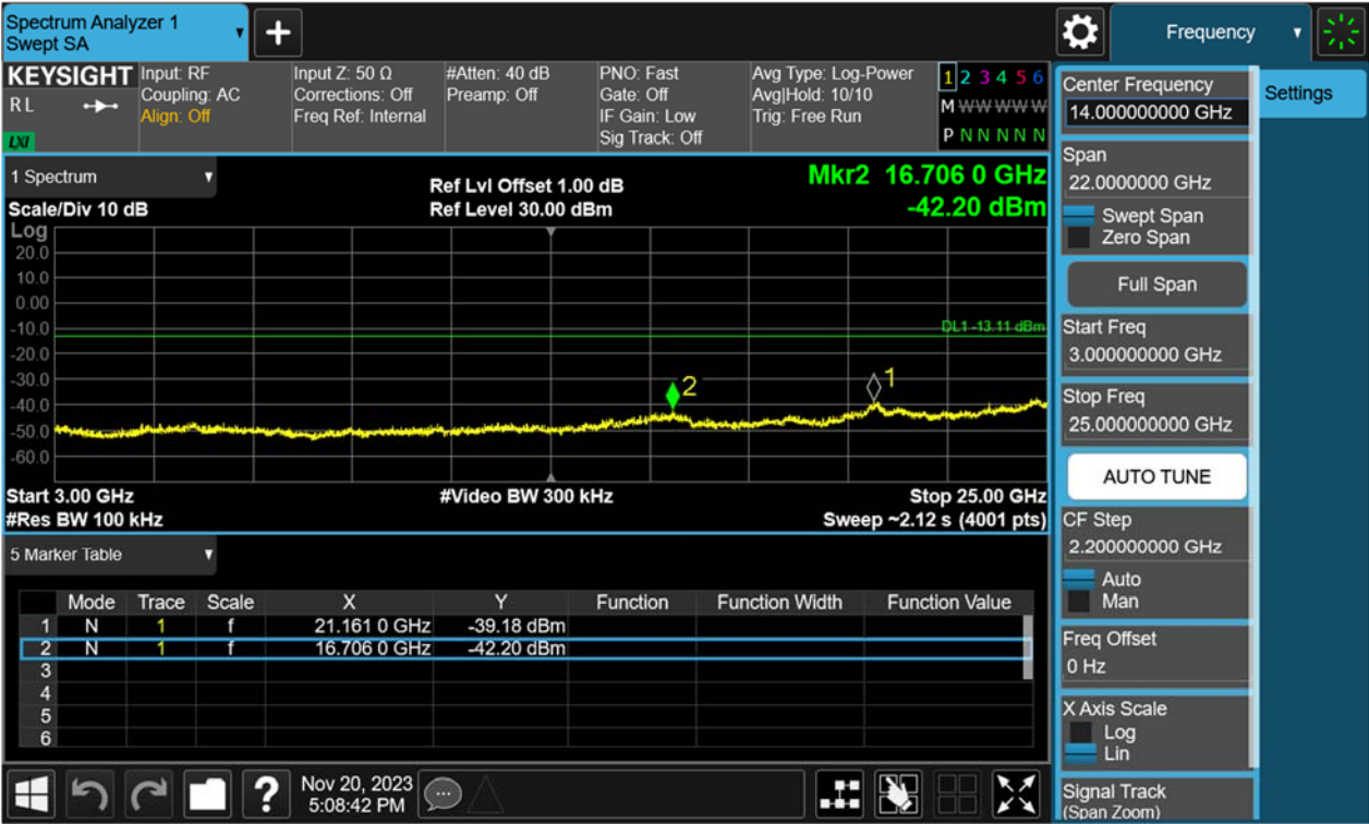
Figure 27: Conducted Spurious Emission & Authorized-band band-edge, 2480MHz, 8-DPSK Carrier Level
