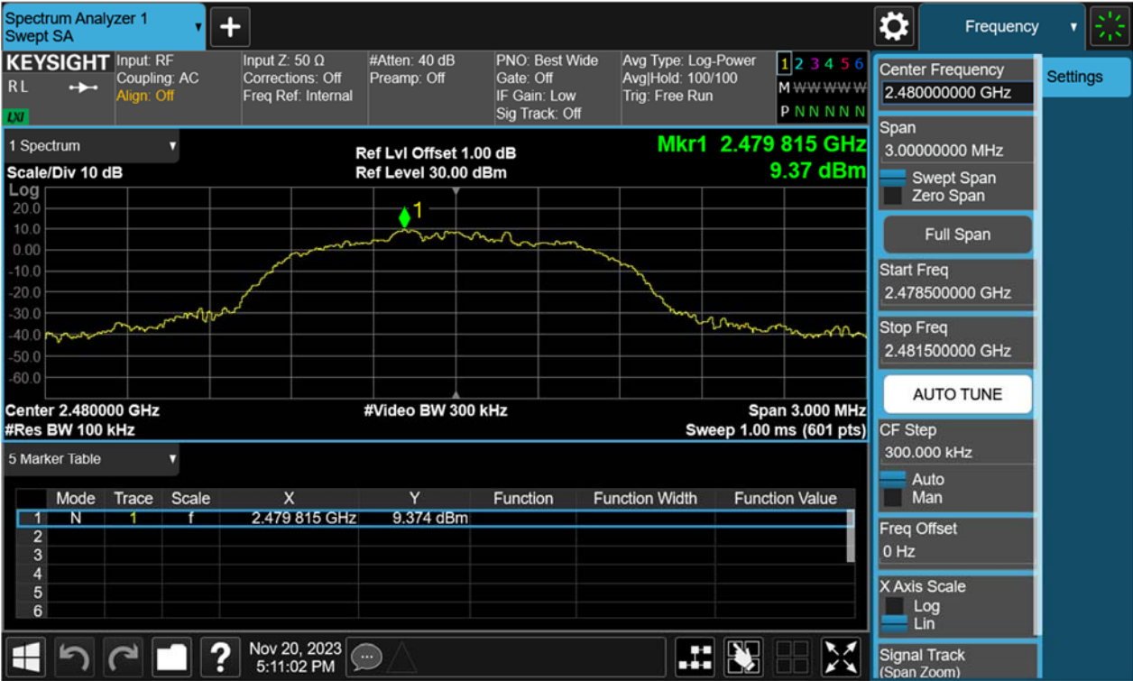
Figure 27: Conducted Spurious Emission & Authorized-band band-edge, 2480MHz, 8-DPSK Carrier Level
