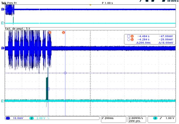
This plot provides a zoom-in to show the 200 ms time interval after the radar burst.
