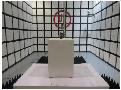
2. RADIATED RF MEASUREMENT SETUP (30MHz~1GHz)
