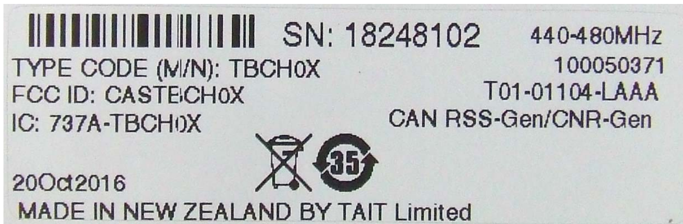
Photograph 03: H2 (440-480 MHz) Reciter module – Compliance label
