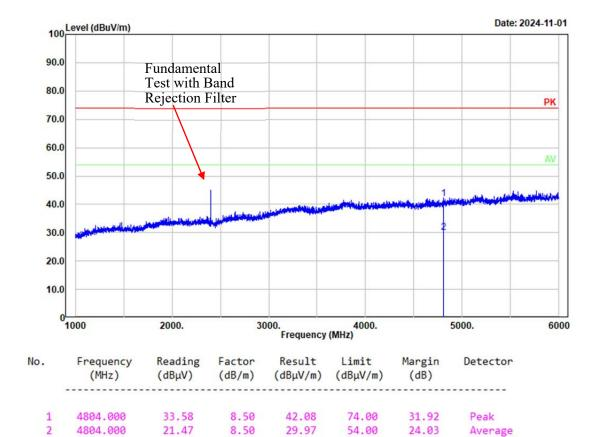
Polarization: vertical Note: BLE 1M Low Channel 2402MHz Chain 0
