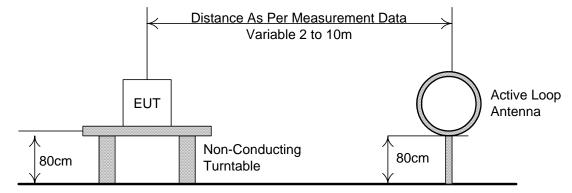
**Test Site For Radiated Emissions Above 30MHz**
