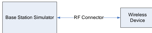
Figure 9-2 Power Measurement Setup
