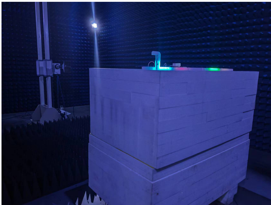
Photo of Radiated Emission Measurement (Above 1G)
