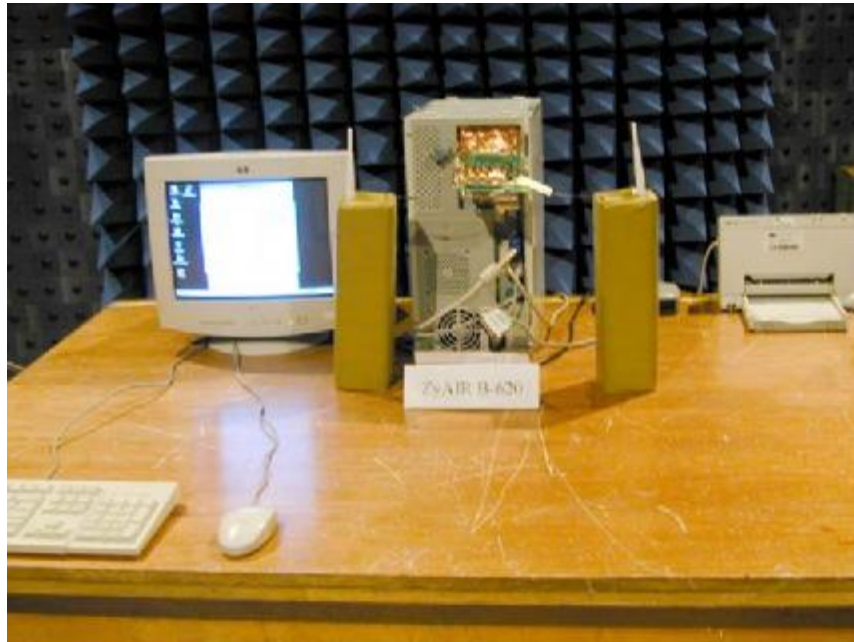
Photo 1: Spurious test set-up photo (front)
