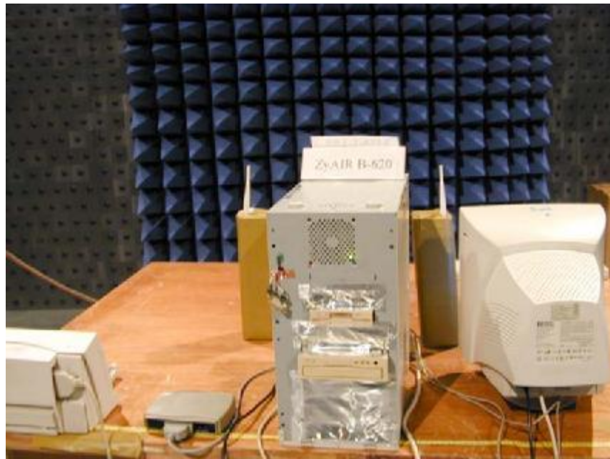
Photo 2: Spurious test set-up photo (rear)
