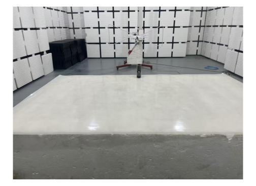
Set-up for Radiated Spurious Emission, Below 1GHz
