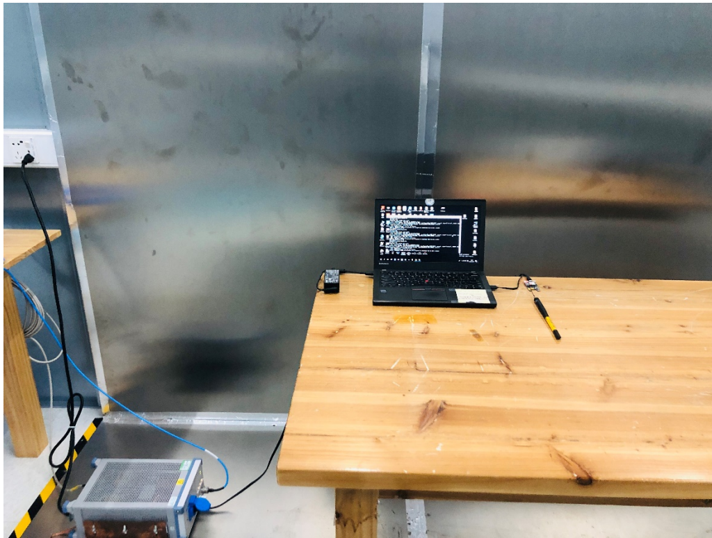
Photograph 3: Set-up for Conducted Emission on AC mains
