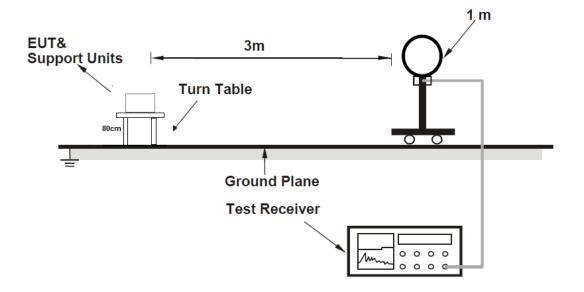
For Radiated emission between 30MHz~1000MHz
