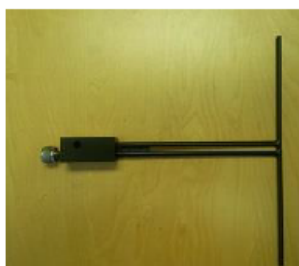
Figure 1 – MVG COMOSAR Validation Dipole
