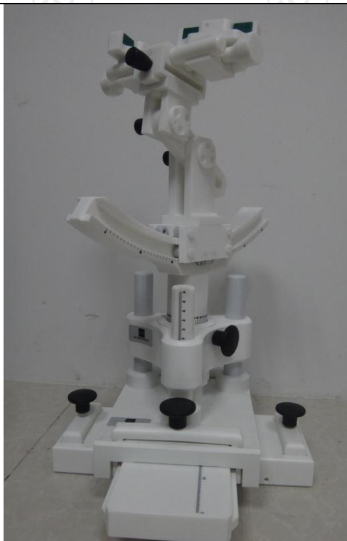
COMOSAR Mobile phone positioning system
