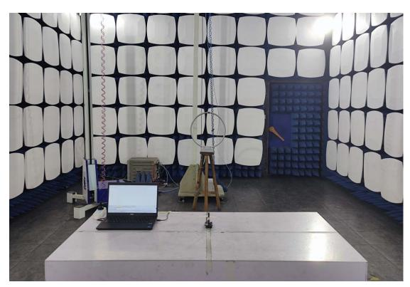
3. Radiated emission (9KHz-30MHz)
