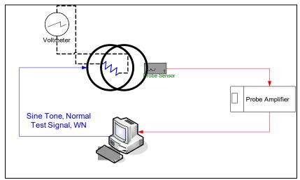
Figure 4-1 Validation Setup with Helmholtz Coil
