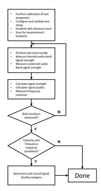
Figure 4-13 C63.19 T-Coil Signal Test Process
