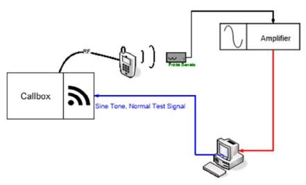
Figure 4-2 **T-Coil Test Setup**
