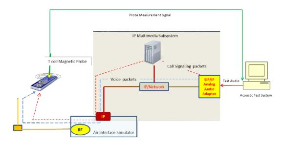
Figure 7-1 Test Setup for VoWIFI over IMS T-Coil Measurements
