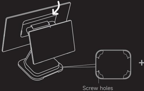
The base screw holes are used to fix the cash drawer.
