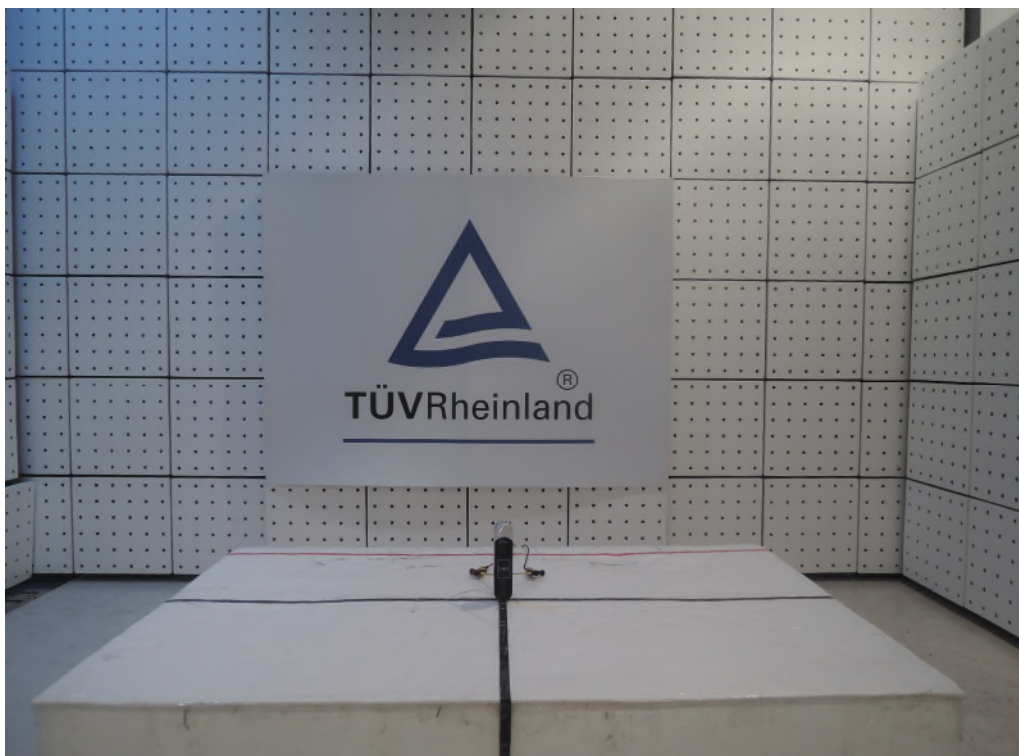
Photograph 2: Set-up for Radiated Emissions (Back View 1)
