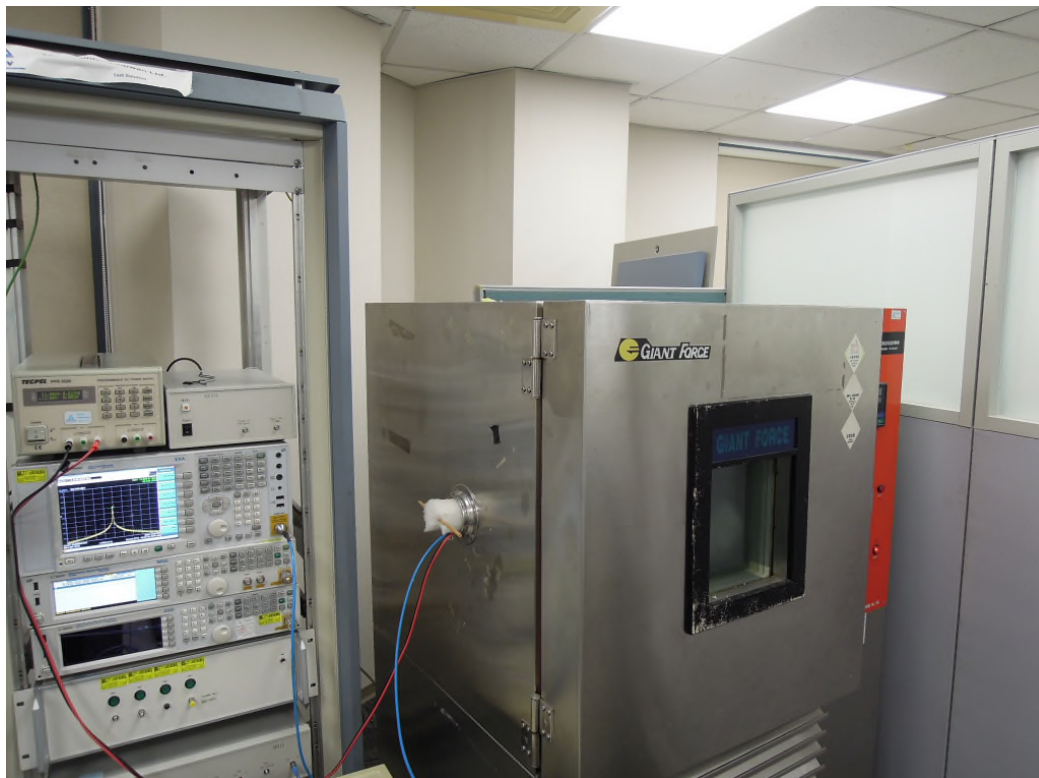
Photograph 4: Set-up for for Conducted testing
