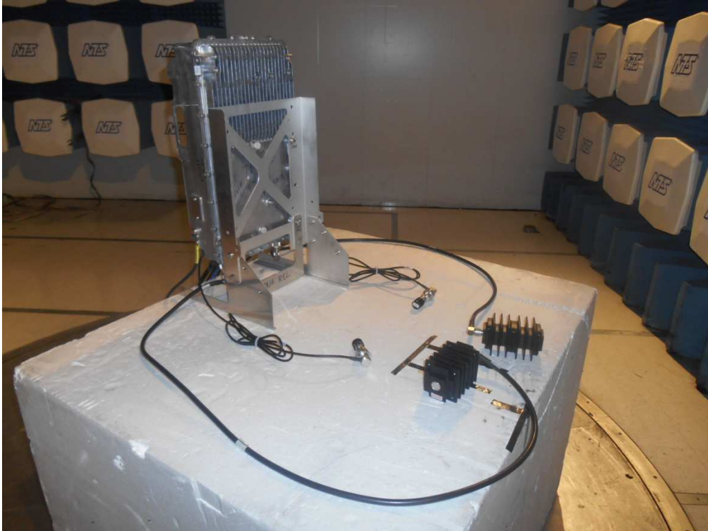
Radiated Emissions Setup – Rear
