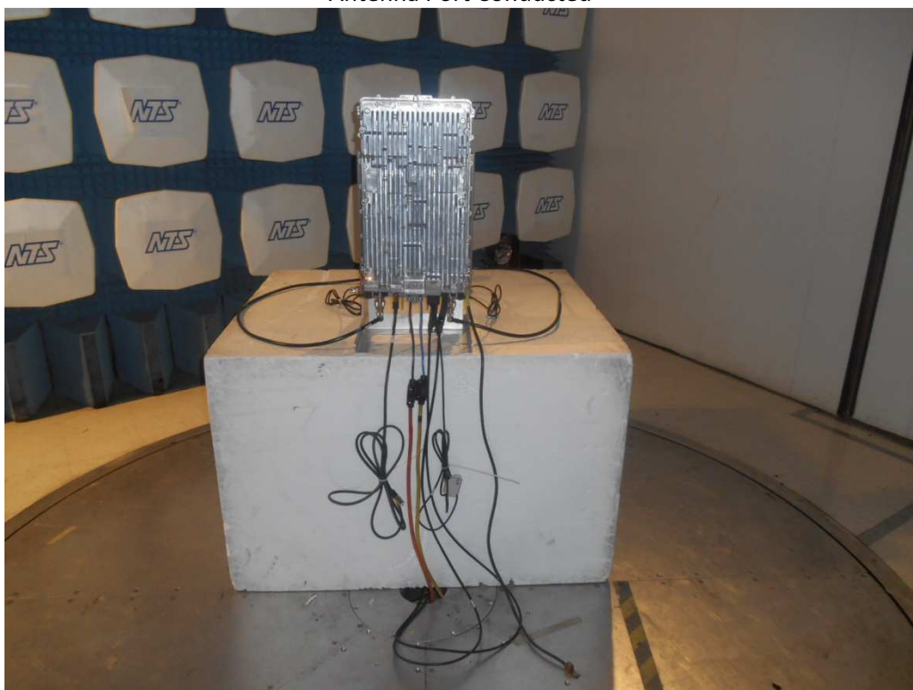
Radiated Emissions Setup - Front
