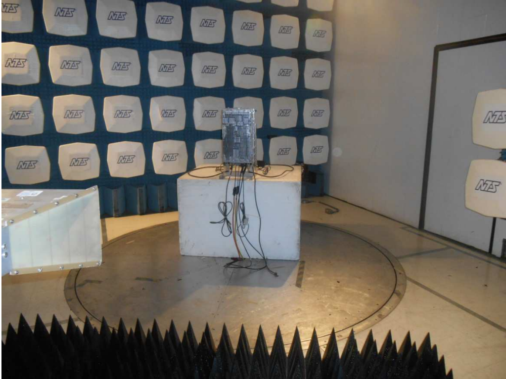
Radiated Emissions Setup – 1GHz to 9GHz
