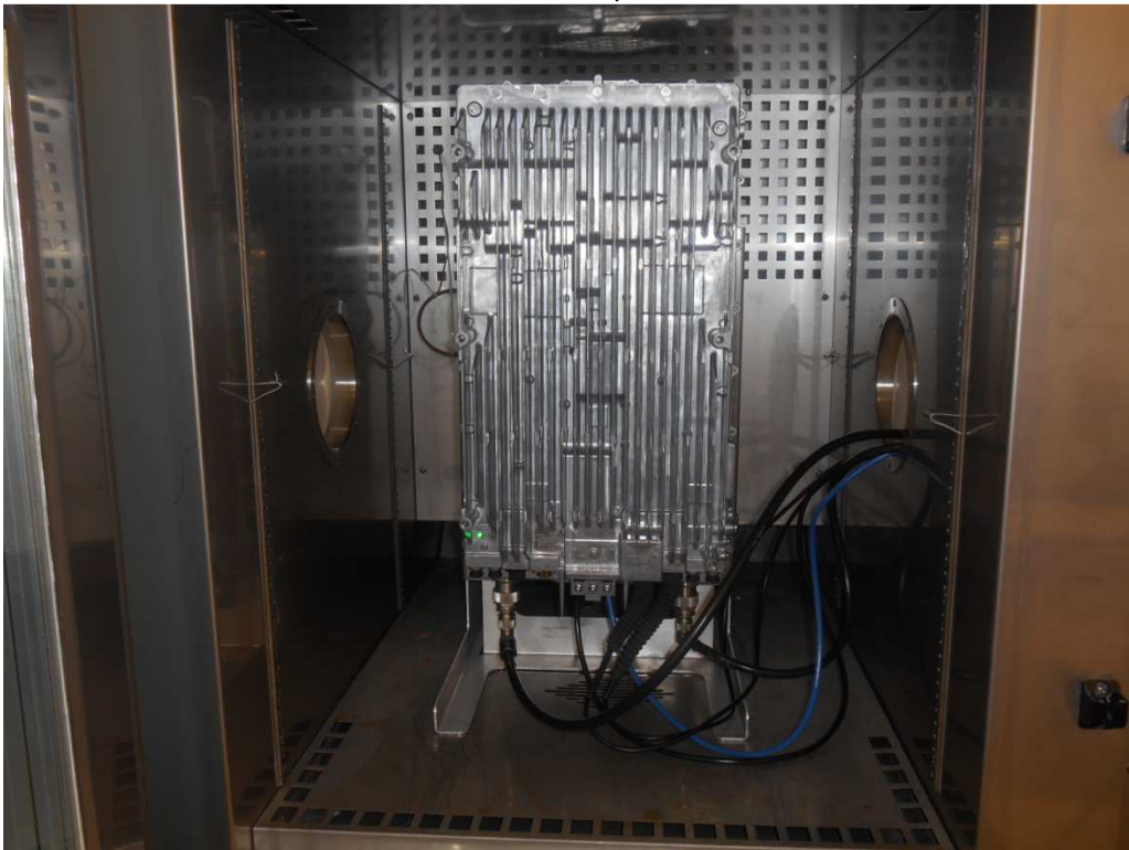
Frequency Stability Setup
