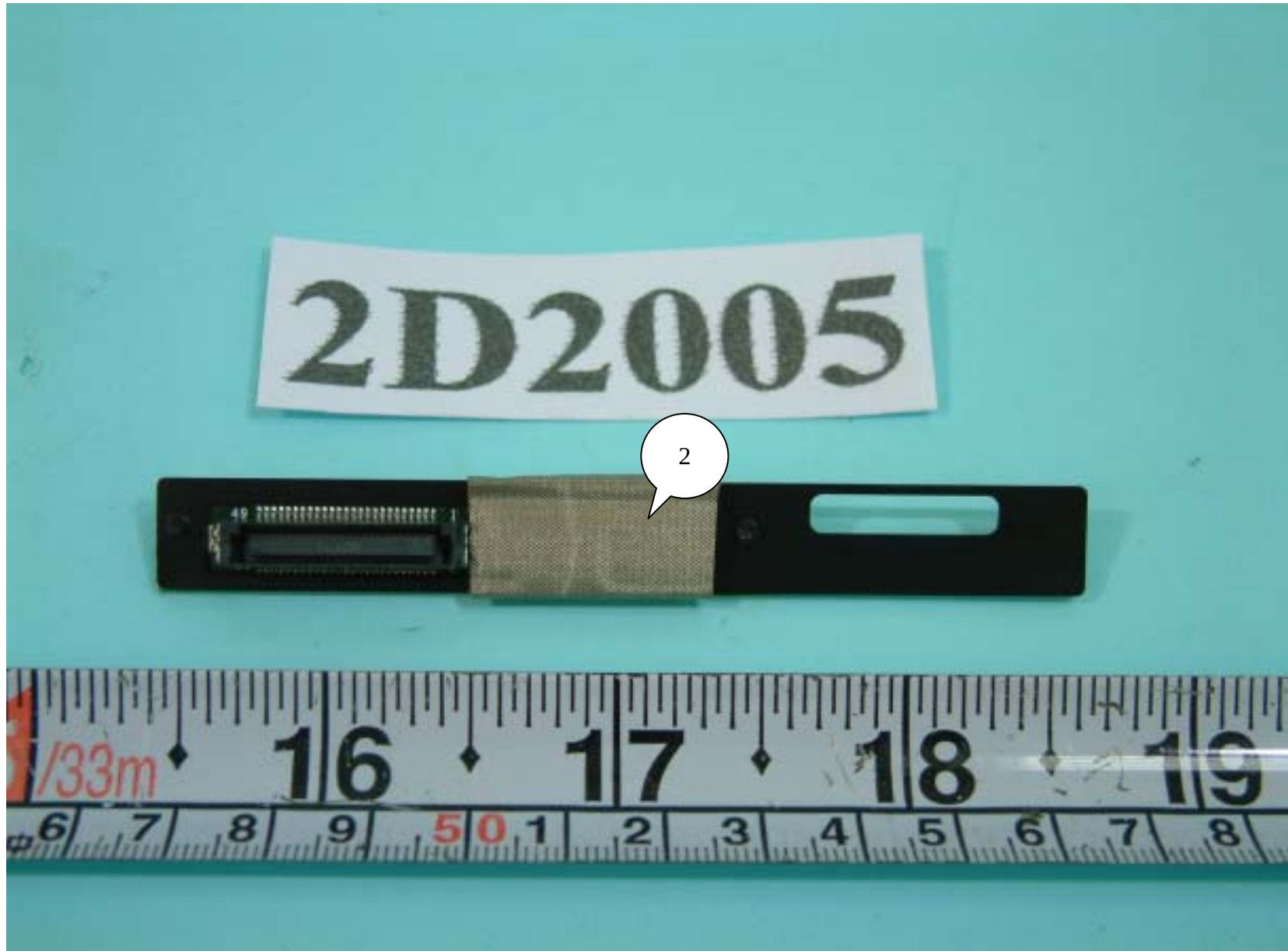
Rear side of CD-ROM connected board
