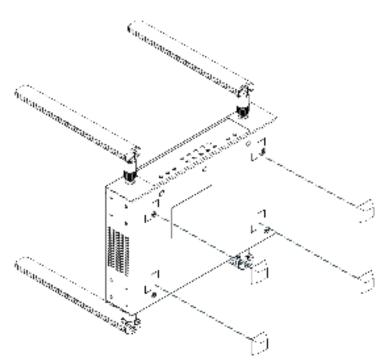
6.2 <u>How to Assemble Unit for RackMounting Using Rack Ears</u>
