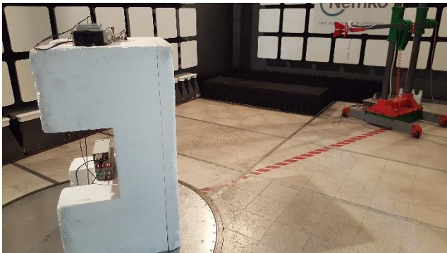
Figure 9.1-3: Radiated setup photo above 1 GHz
