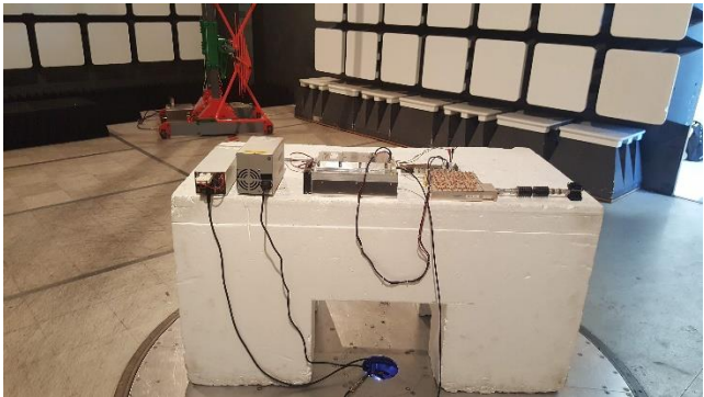
Figure 9.1-2: Radiated setup photo below 1 GHz
