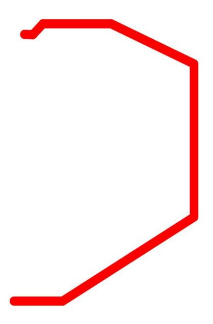
Remote control antenna specification Antenna size: 433M, antenna, material: Copper The antenna is whip with a width of 0.8mm a thickness of 1 oz and a total straightening length of 45mm Antenna Gain: OdBi
