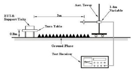
The radiated emission tests were performed in the 3 meters chamber, using the setup accordance with the ANSI C63.4-2014. The specification used was with the FCC Part 15 B Class B limits.
