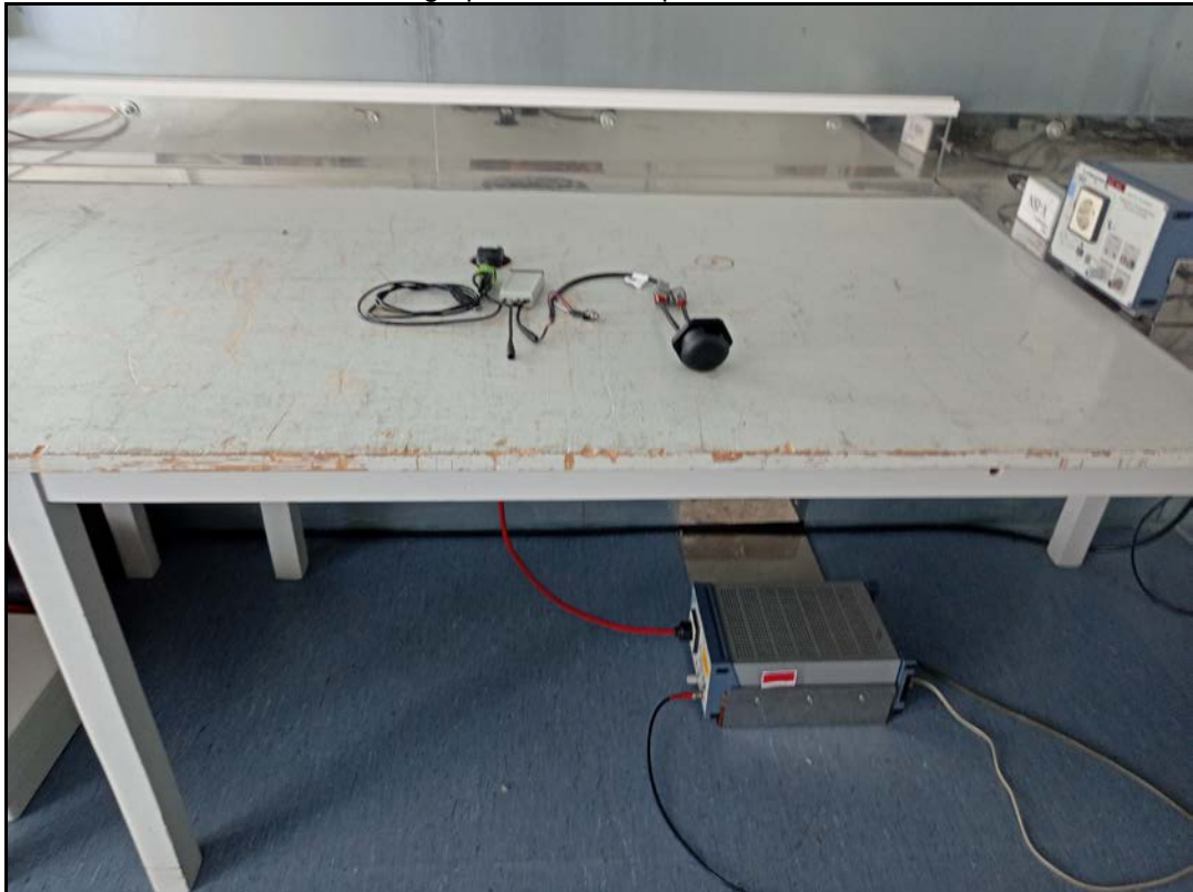
Photo 1: Photograph of Test setup 1 conducted emission
