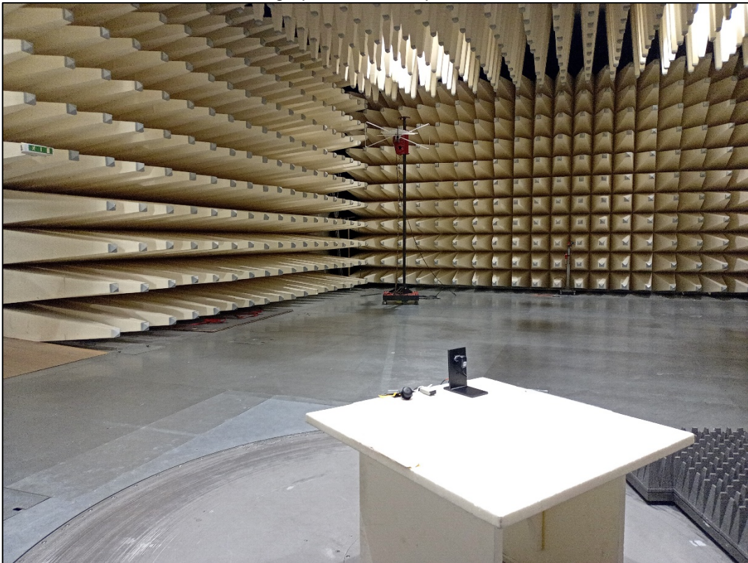
Photo 5: Photograph of Test setup 2 radiated emission
