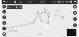
The aircraft will fly automatically to the first waypoint, the second one, the third one and so on by pressing the "One-key waypoint take-off" on the remote control after setting. Then, the aircraft will be hovering for standby at the last waypoint. After that, please click to delete the set waypoints
