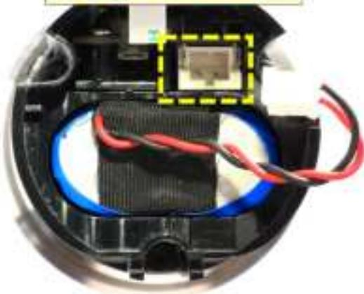
Confirm the battery connector, "black line on left, red line on right"
