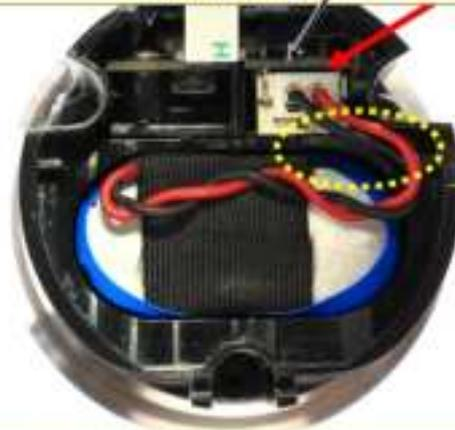
Place the cable inside the groove, ensuring it does not protrude. This prevents the cable from being pinched or the cover from lifting when the cover is closed.
