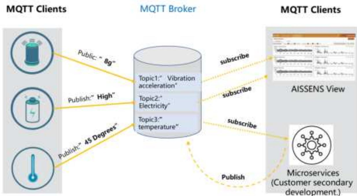
MQTT (Message Queuing Telemetry Transport) is a lightweight communication protocol commonly used for data transmission between Internet of Things (IoT) devices. It is based on the publish/subscribe model and is suitable for scenarios with limited network bandwidth. The MQTT architecture consists of three parts: Publisher, Broker, and Subscriber.
