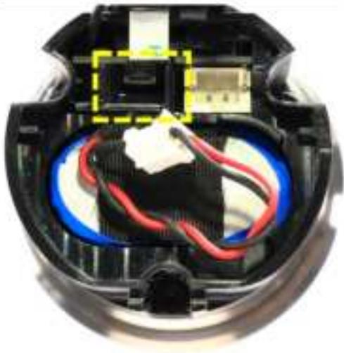
Place the cable inside the groove, ensuring it does not protrude. This prevents the cable from being pinched or the cover from lifting when the cover is closed.
