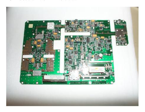
PCB inside the LNA/PA – Back View
