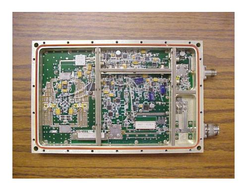
**GDL RF Assembly Component with Housing Close View**
