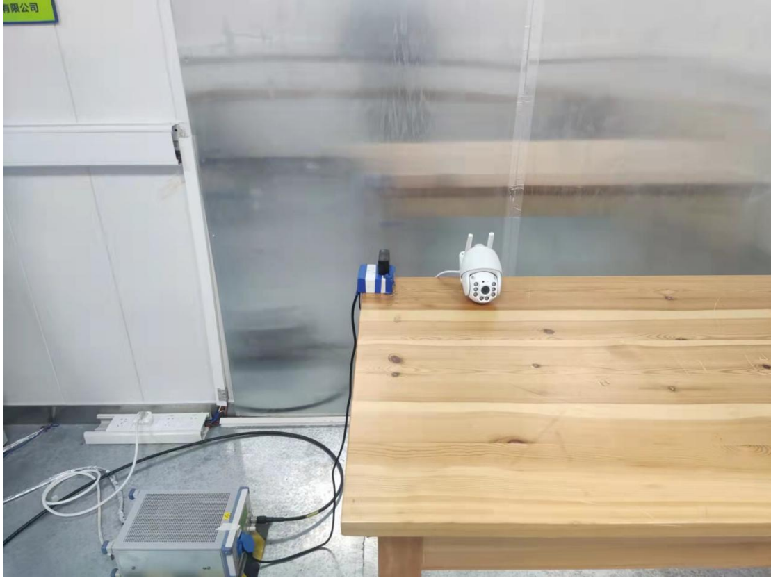
Conducted emission test setup
