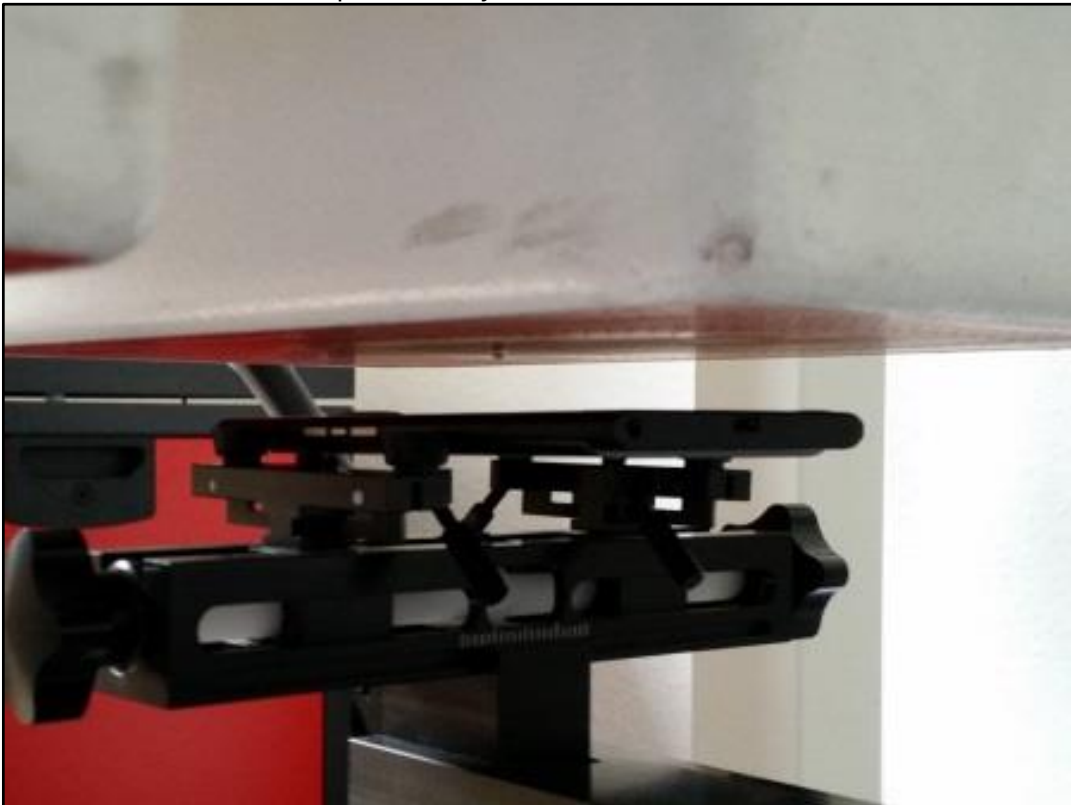
Photo 40: Test position body worn rear side with 15 mm distance
