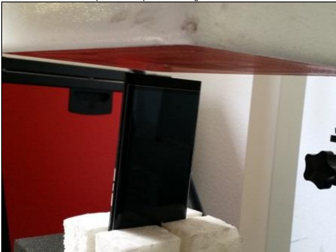
Photo 32: Test position hotspot bottom edge side with 10 mm distance
