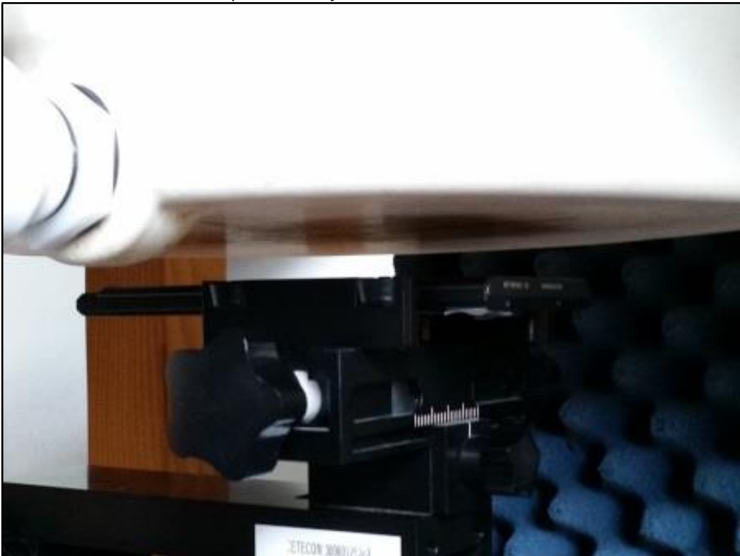
Photo 41: Test position body worn front side with 15 mm distance
