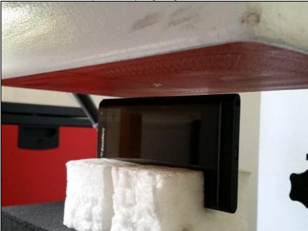
Photo 30: Test position hotspot right edge side with 10 mm distance
