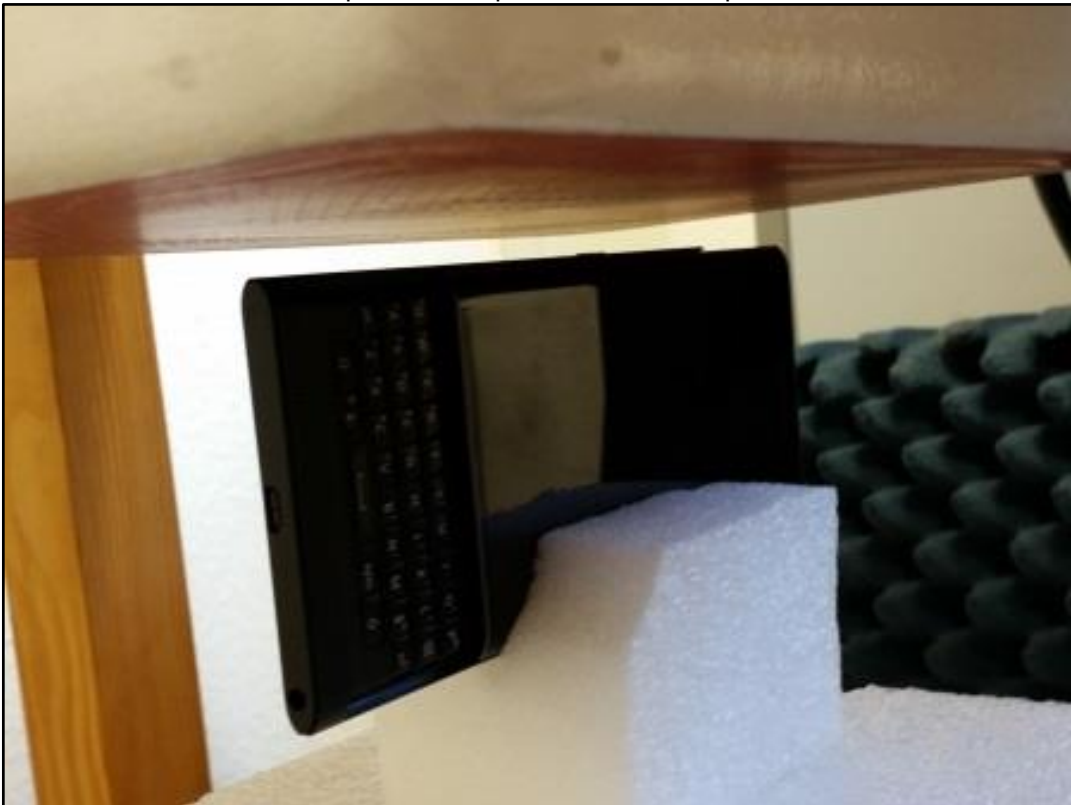
Photo 35: Test position hotspot left side slider open with 10 mm
