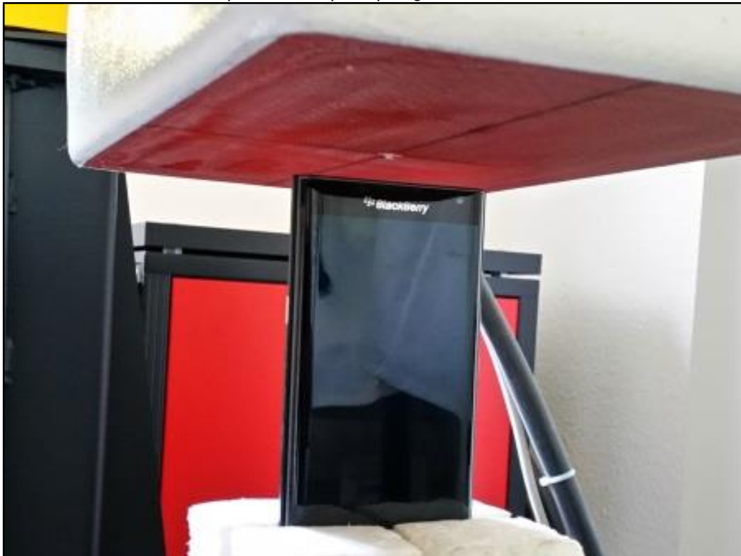
Photo 31: Test position hotspot top edge side with 10 mm distance
