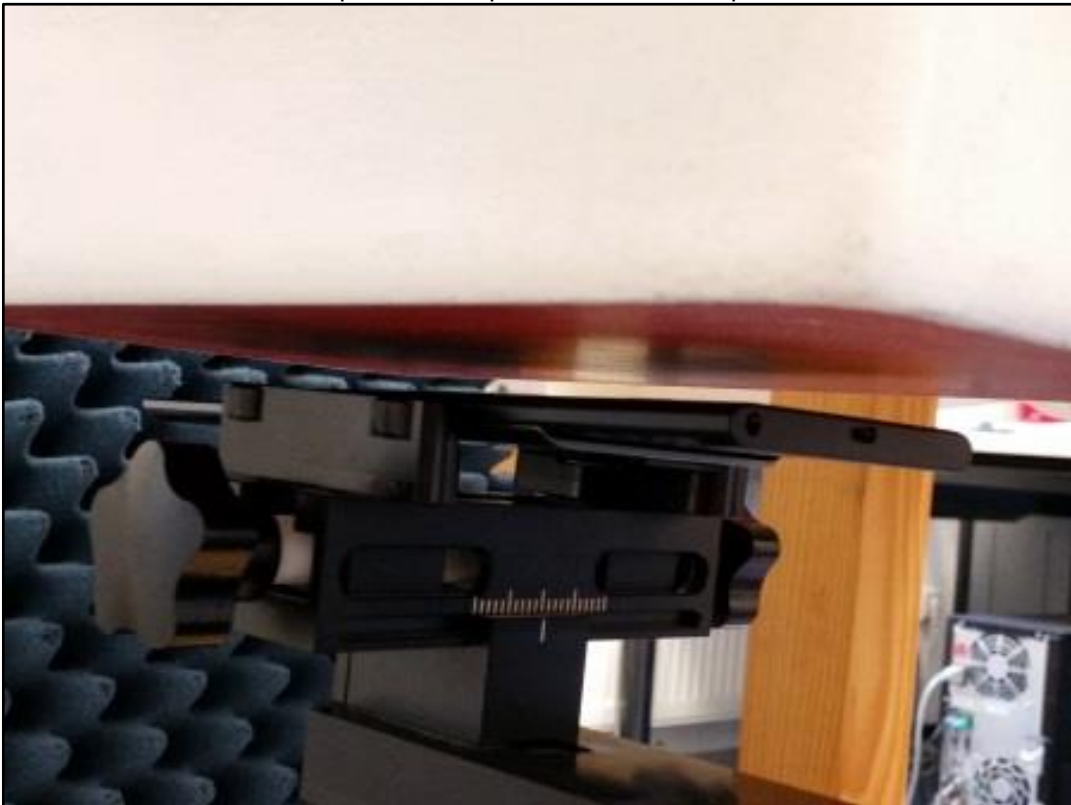
Photo 34: Test position hotspot rear side slider open with 10 mm
