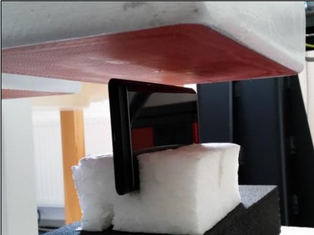
Photo 29: Test position hotspot left edge side with 10 mm distance
