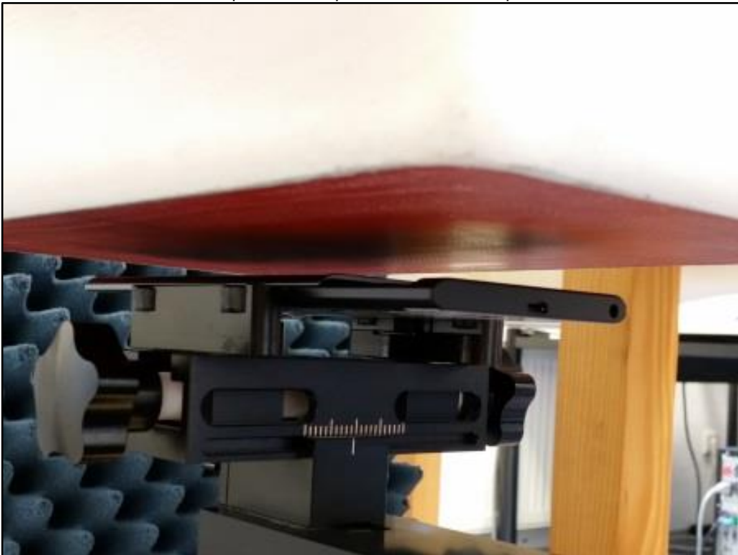
Photo 33: Test position hotspot front side slider open with 10 mm
