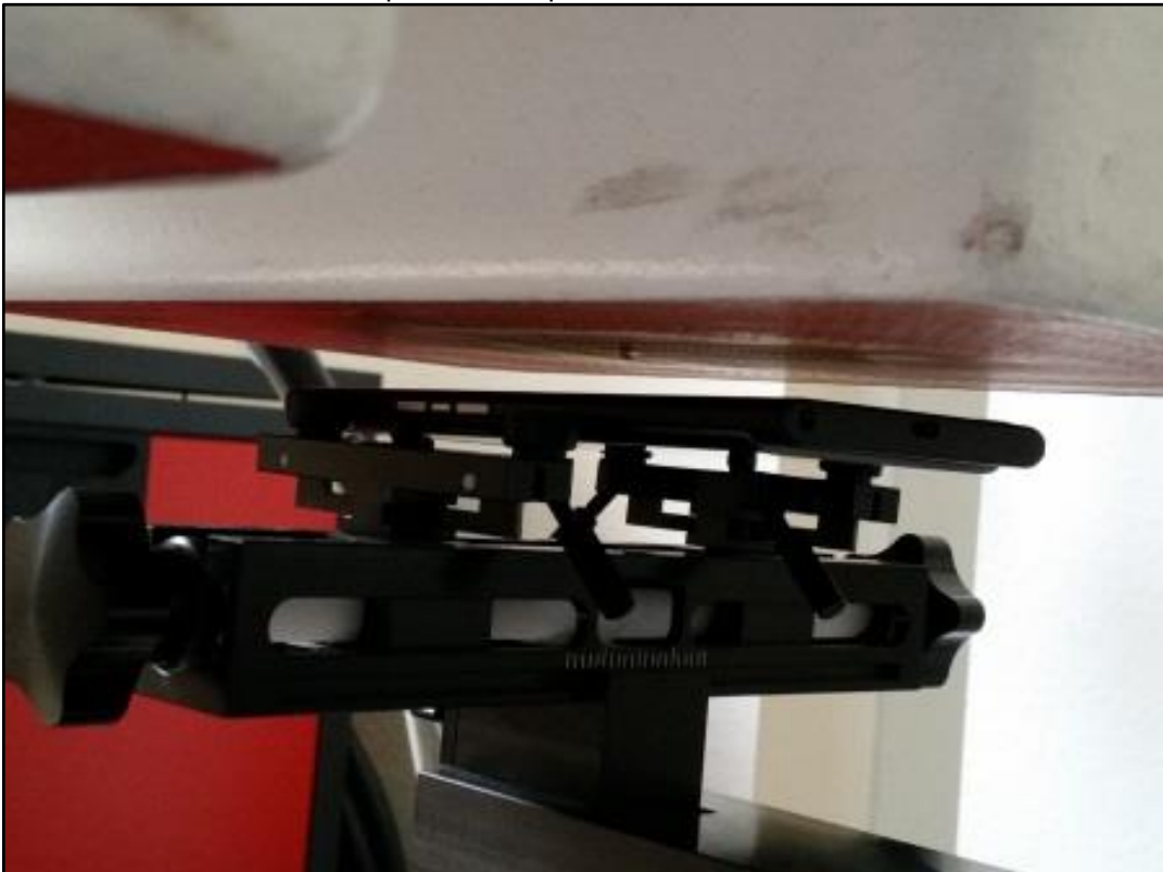
Photo 28: Test position hotspot rear side with 10 mm distance
