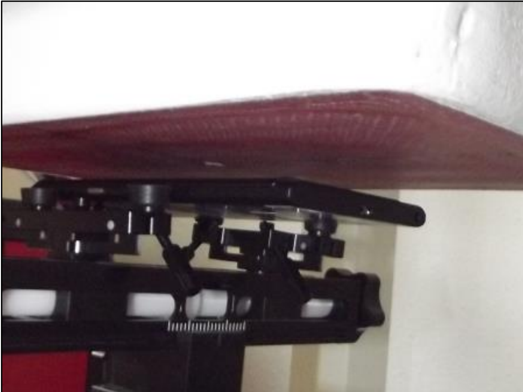
Photo 27: Test position hotspot front side with 10 mm distance
