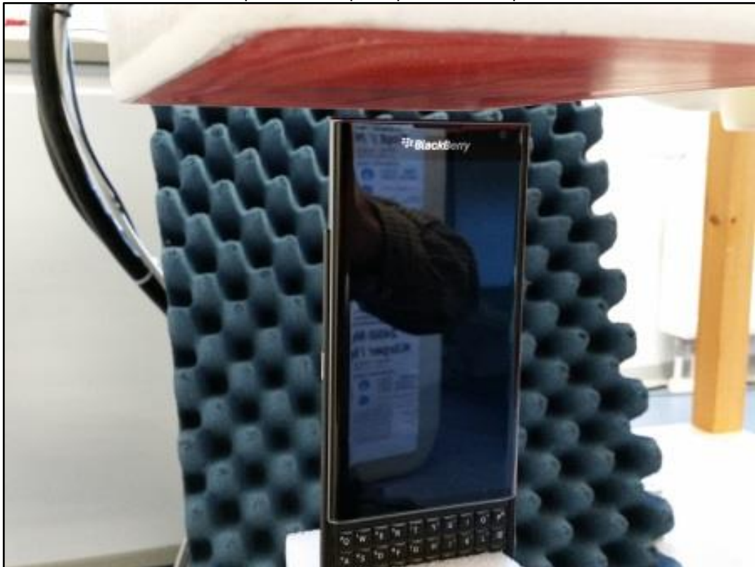
Photo 37: Test position hotspot top side slider open with 10 mm
