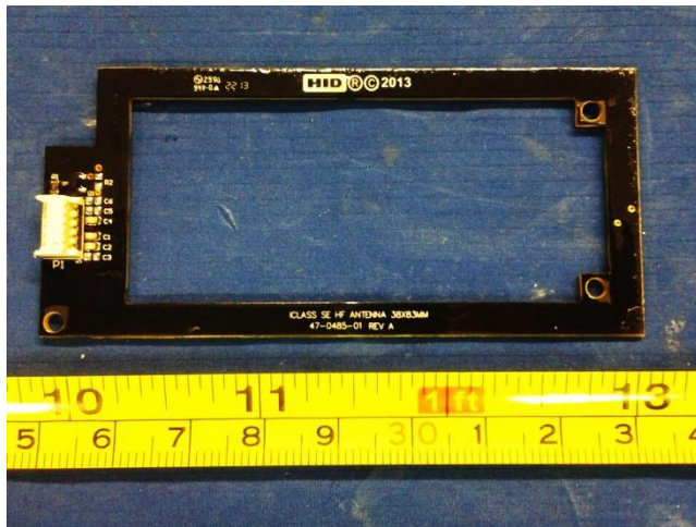
High Frequency Long Antenna Top View
