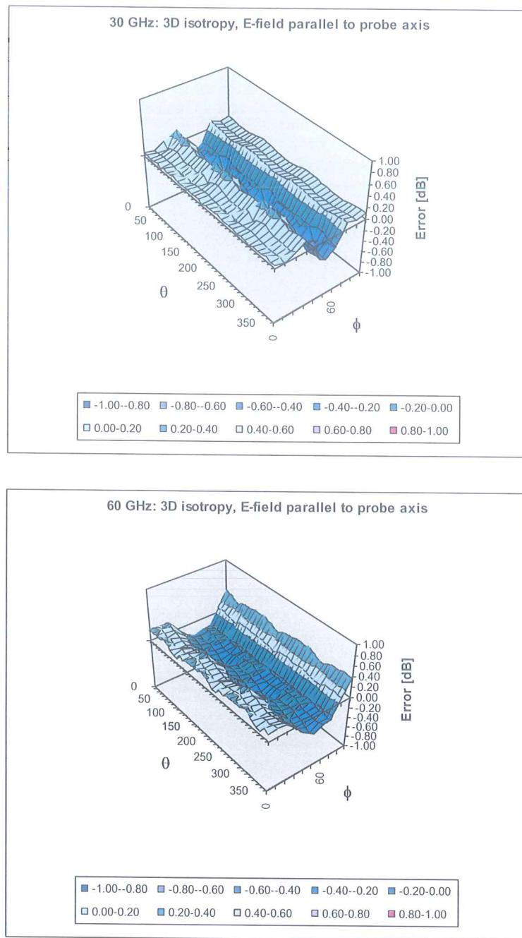
Probe isotropy for  $E_{\text{tot}}$ : probe rotated  $\varphi = 0^\circ$  to  $360^\circ$ , tilted from field propagation direction  $\vec{k}$
