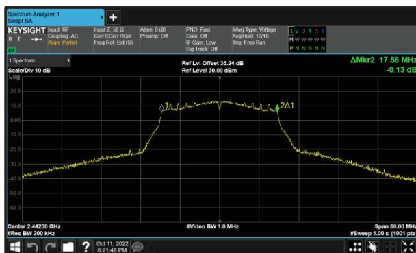
Figure 43 - 802.11n HT20 Minimum 99% OBW
