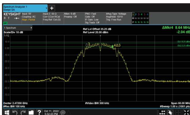
Figure 31 - 802.11b Minimum 6 dB EBW
