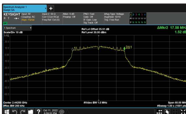
Figure 51 - 802.11n HT20 Minimum 99% OBW
