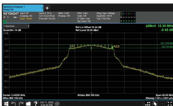
Figure 33 - 802.11g Minimum 6 dB EBW
