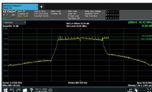
Figure 49 - 802.11ax HE20 SU Minimum 6 dB EBW
