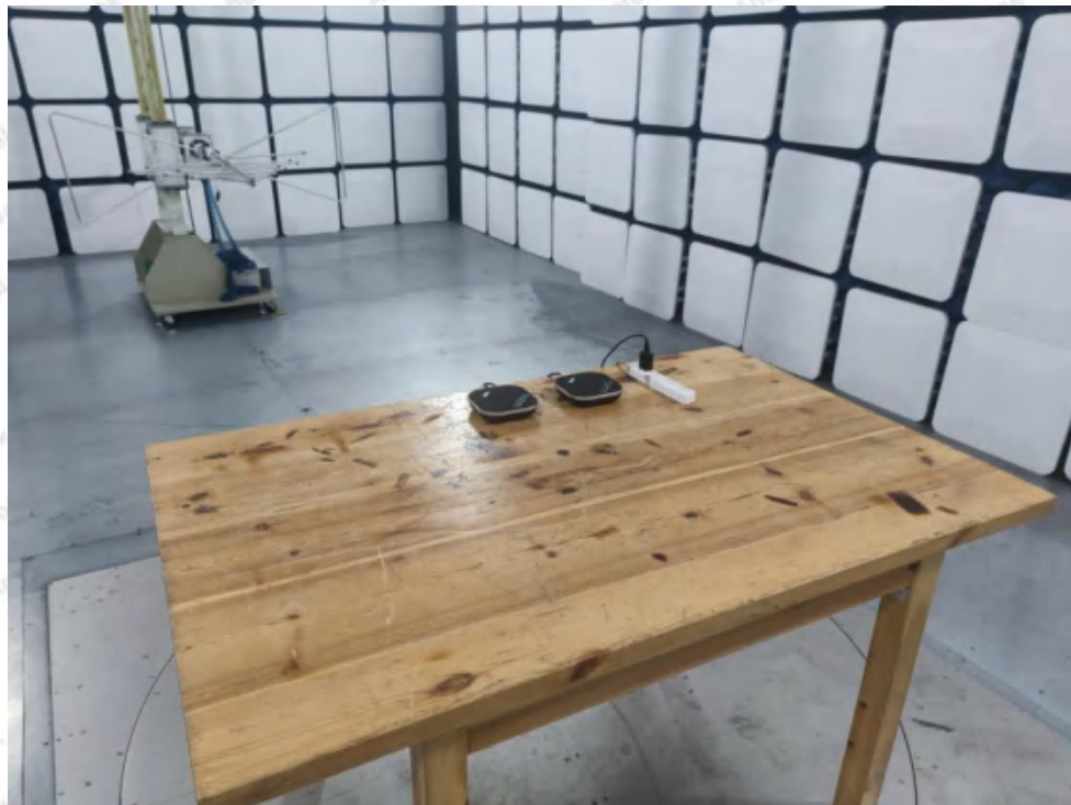
Photo of Radiation Emission Test
