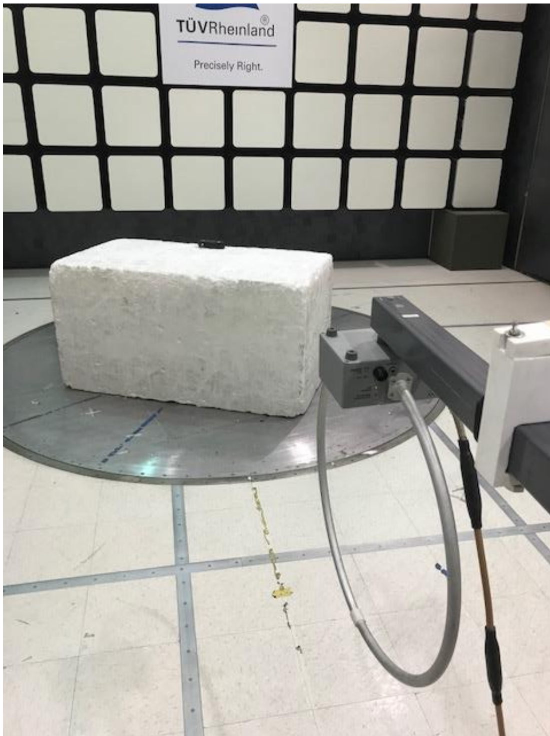
Test setup 9k to 30M Front
