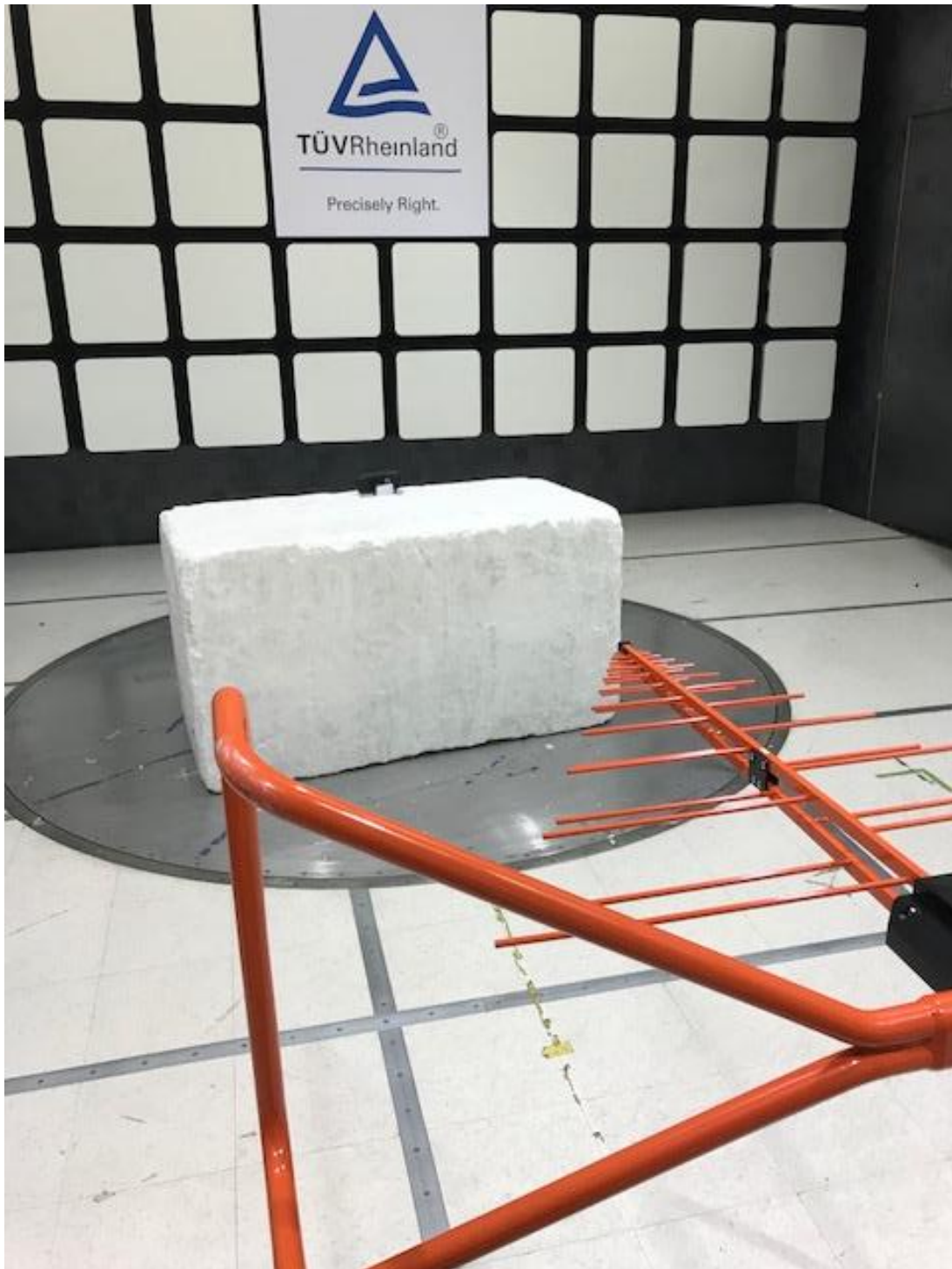
Test Setup 30-1000M Front
