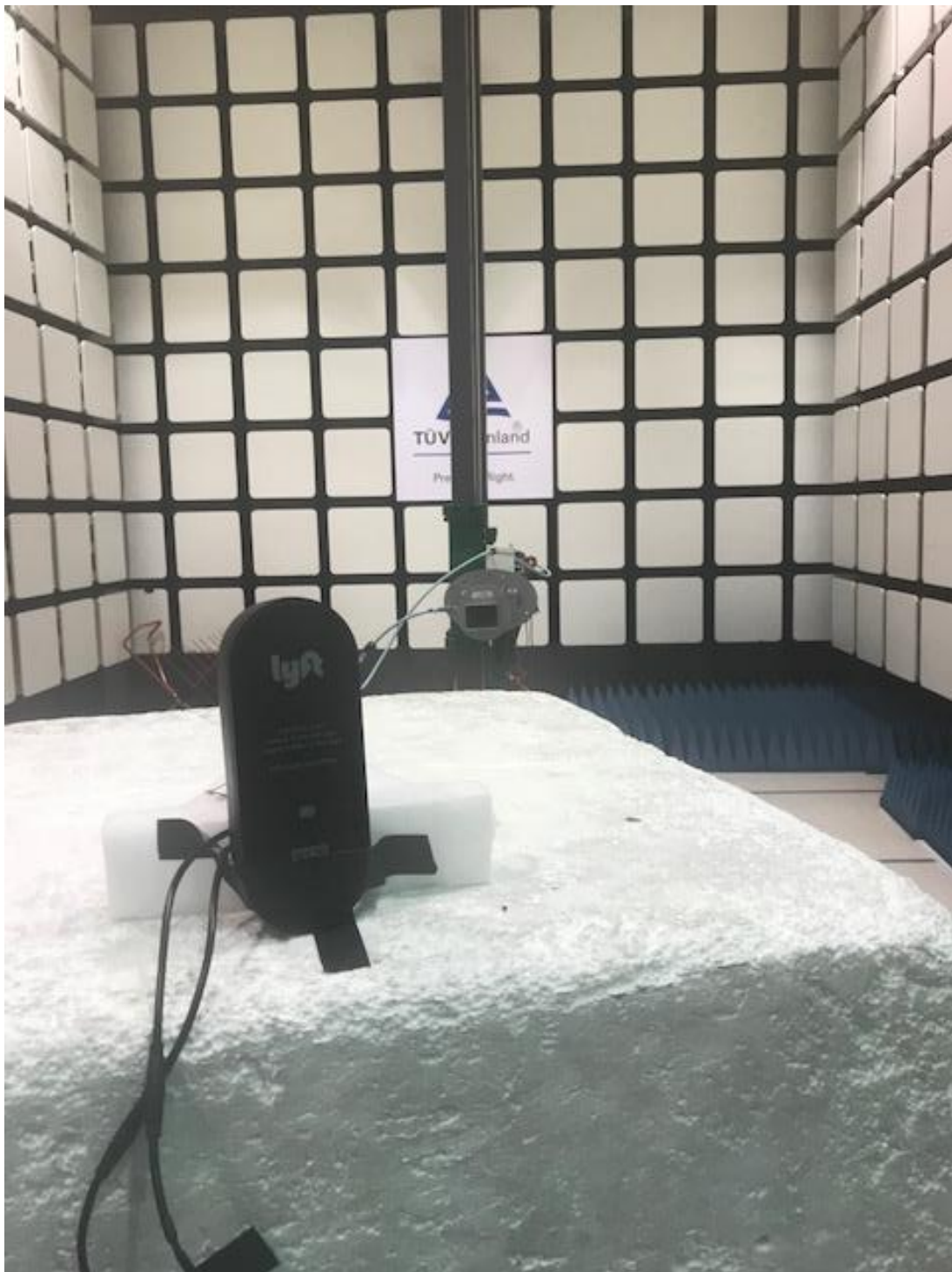
Test Setup 18-26G Rear
