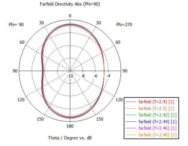
The figure below illustrates the energy radiation cross-sectional diagram in the XOZ plane, where different colors correspond to distinct frequencies. The frequency represented by each color can be identified via the description in the lower-right corner of the graph. For instance, the first row labeled "Red F=2.4" denotes a frequency of 2.4 GHz. The energy radiation pattern can be referenced to the circular diagram for reference.
