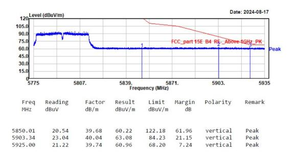
Project No.: 2407W89604E-RF Test Mode: 11ac80-5775 EUT Model: SLM927 Test distance: 3m Temp/Humi/ATM: 23.9℃/60%/100.1kPa Tested by: Wlif Wu Power Source: AC 120V/60Hz
