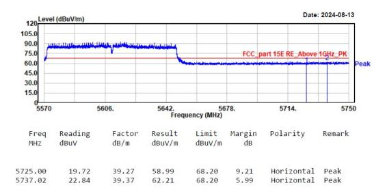
Project No.: 2407W89604E-RF Test Mode: 11ac80-5610 EUT Model: SLM927 Test distance: 3m Temp/Humi/ATM: 23.9℃/60%/100.1kPa Tested by: Wlif Wu Power Source: AC 120V/60Hz
