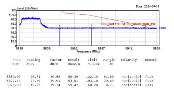
Project No.: 2407W89604E-RF Test Mode: 11a-5825 EUT Model: SLM927 Test distance: 3m Temp/Humi/ATM: 23.9°C/60%/100.1kPa Tested by: Wlif Wu Power Source: AC 120V/60Hz
