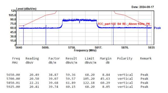
Project No.: 2407W89604E-RF Test Mode: 11ac80-5775 EUT Model: SLM927 Test distance: 3m Temp/Humi/ATM: 23.9°C/60%/100.1kPa Tested by: Wlif Wu Power Source: AC 120V/60Hz
