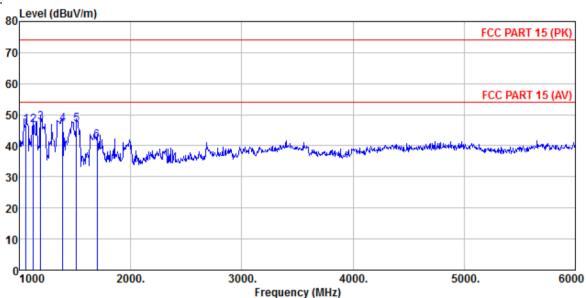
Condition : FCC PART 15 (PK) I Test Mode : Burning test mode Test Engineer: He : FCC PART 15 (PK) BBHA9120D ANT(>1GHZ) VERTICAL
