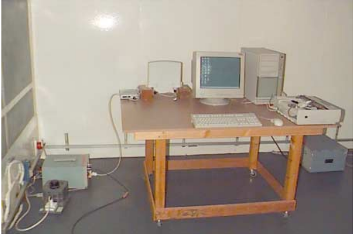
Photograph 4.6.1 Setup view for conducted emission measurements
