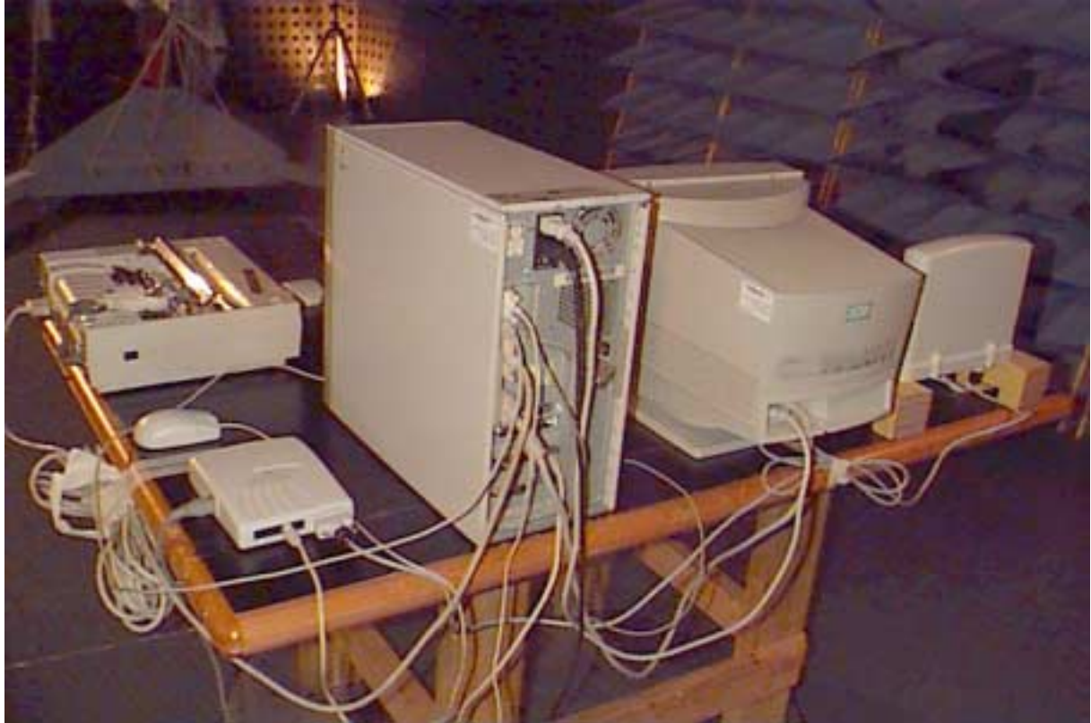
Photograph 4.8.3 Setup for radiated emission measurements, EUT view
