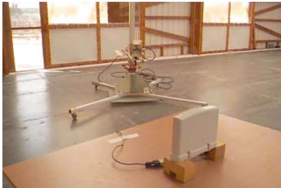
Photograph 4.5.5 Setup for spurious emission field strength measurements in 1 to 7.5 GHz band
