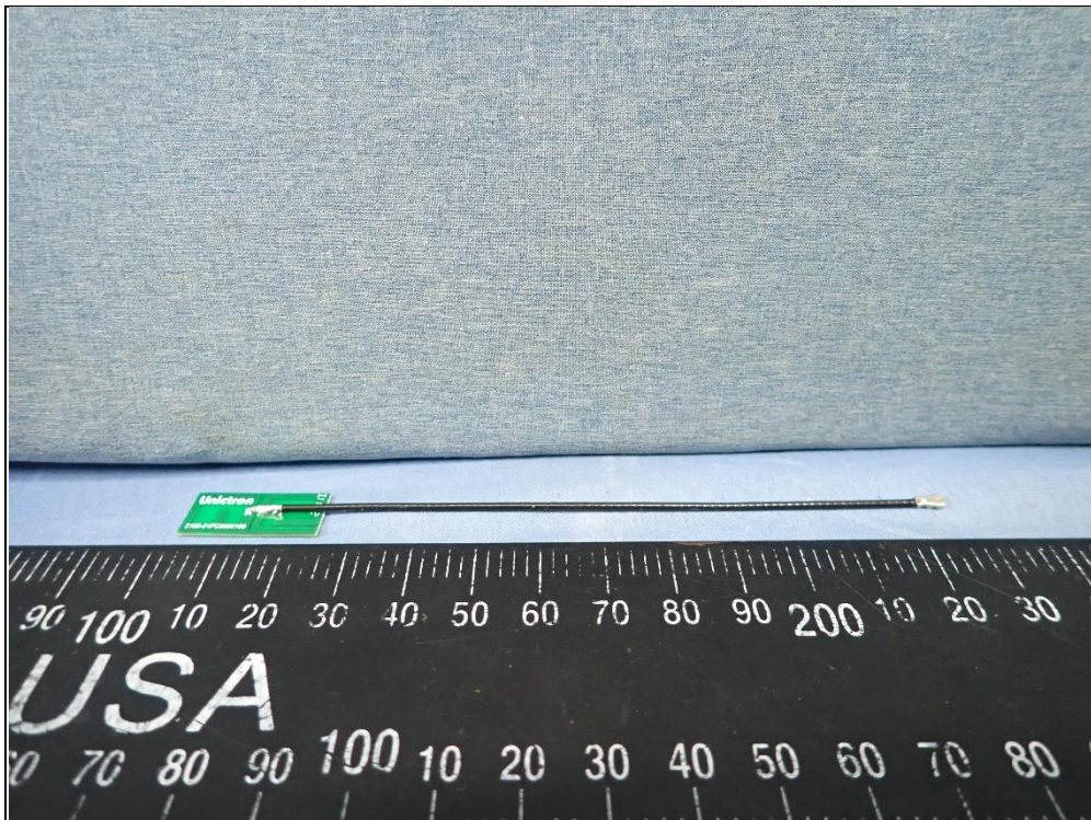
Dipole Antenna (Brand: Unicttron / Model: PC-W09-01)
