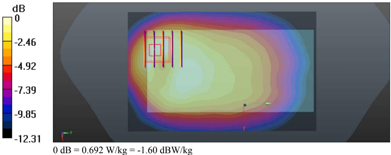
**23\_LTE Band 4\_20M\_QPSK\_1RB\_49Offset\_Bottom Side\_10mm\_Ch20175**
