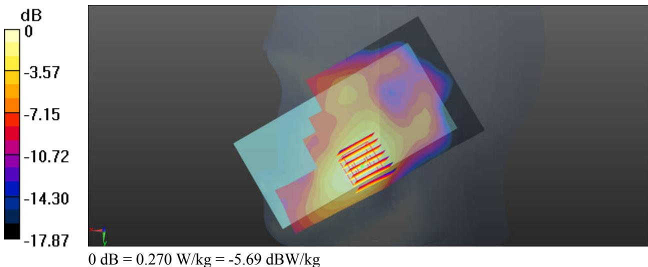
**09\_LTE Band 2\_20M\_QPSK\_1RB\_49Offset\_Right Cheek\_0mm\_Ch19100**
