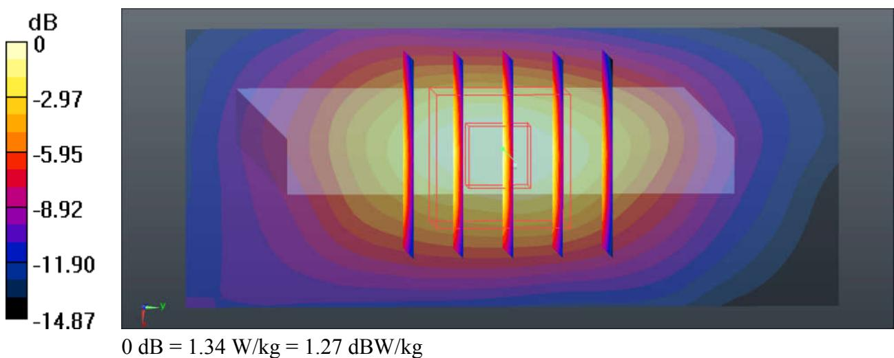
**24\_LTE Band 2\_20M\_QPSK\_1RB\_49Offset\_Bottom Side\_10mm\_Ch19100**
