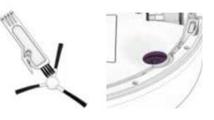
**4.** Clean the main brush and all its components, including the brush gate and brush compartment.
