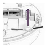
**3.** Pinch the tabs on the main brush gate and lift.
