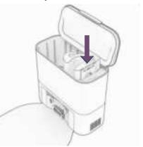
2. Pull up the tab to close the dust bag's opening. Lift to remove the full dust bag and discard.
