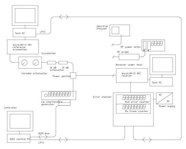
Figure 1, measurement test set-up.
