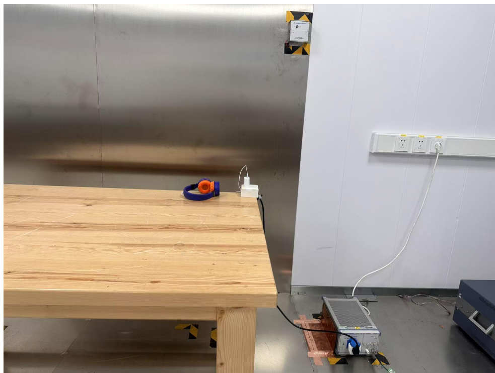
Radiated Emission Test View|(Below 1G)
