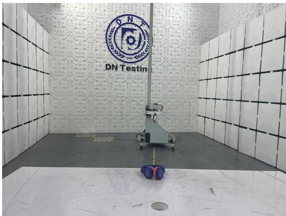
Radiated Emission Test View|(Below 1G)
