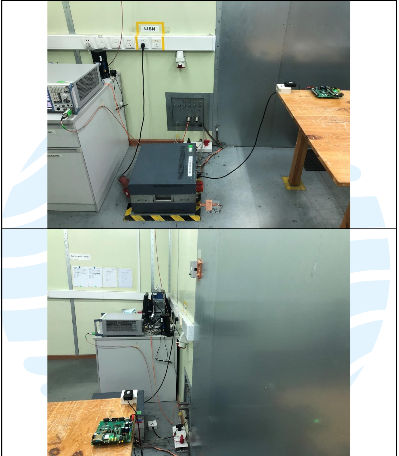
Conducted Emission Test Setup-3
