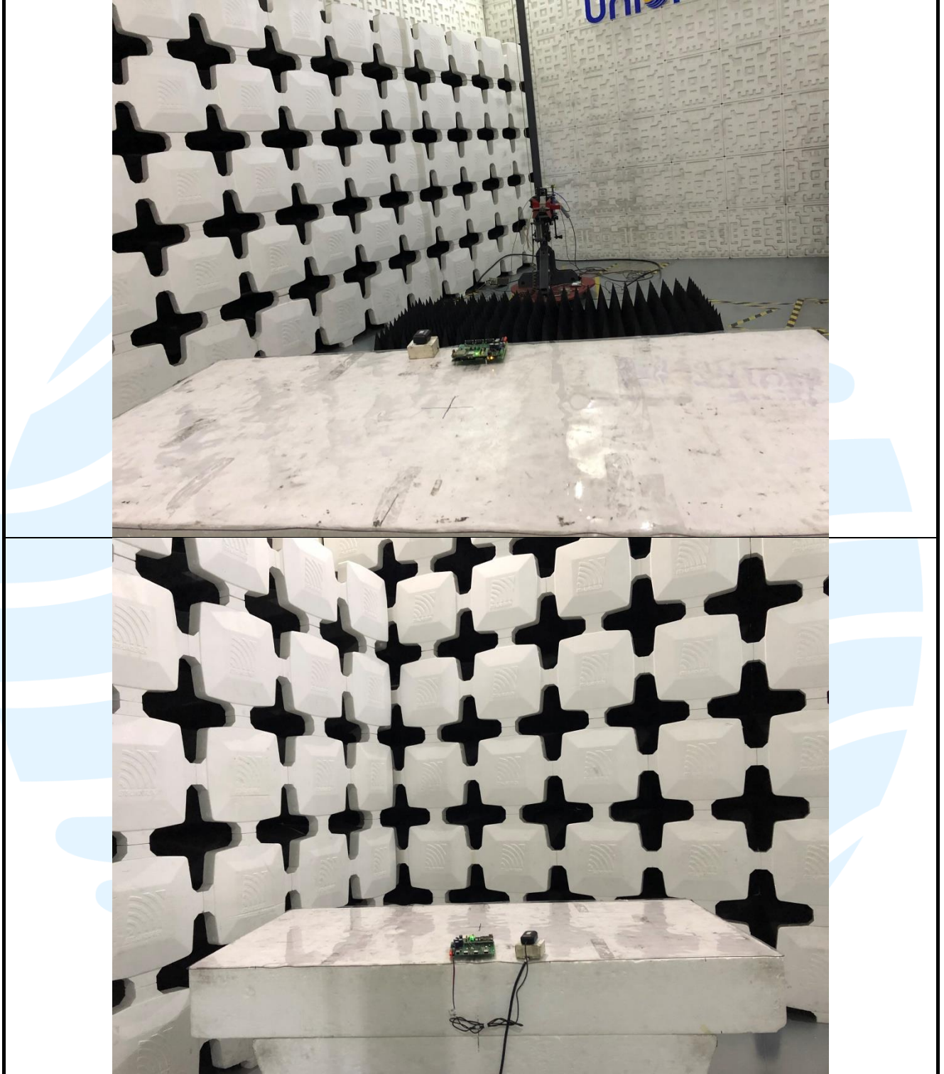
Radiated emission Test Setup-2 (Above 1 GHz)
