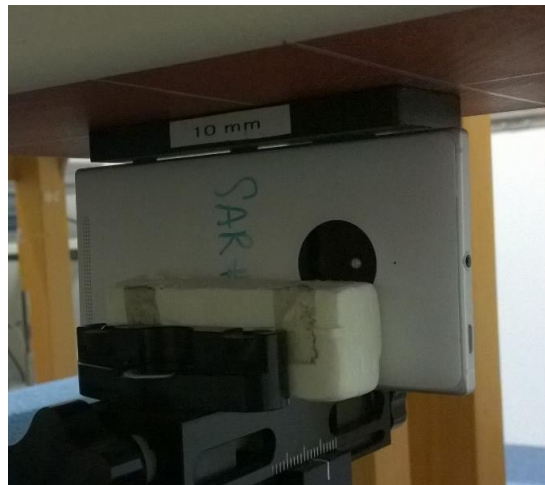
Photo of the device positioned for WR mode measurement – right edge facing phantom. The spacer was removed before the start of the measurements
