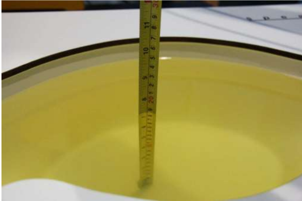
Picture 7-4: Liquid depth in the Head Phantom(2450MHz)
